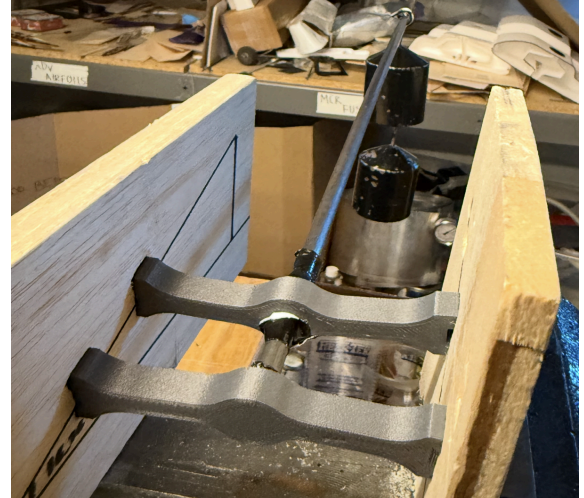
Figure 7.11.3: (left) Shear Force and Bending Moment Graph of Tail Mounts & (right) Weighted Bending Test Setup
